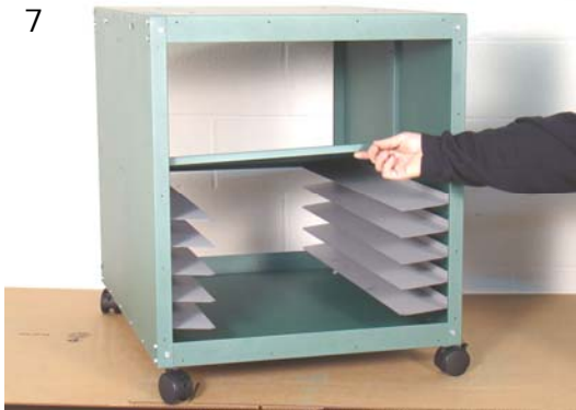
7) Install Utility Shelf onto the top (2) Screen Shelves. Utility Shelf lays on top of the Screen Shelves with it's flanges facing down.
